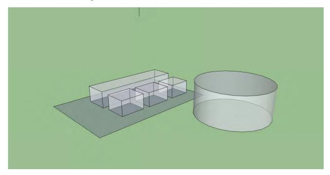
Pool Tank = 684 m3 (existing) Pools 1 to 3 = 300 m3 (new) Tank 4 = 400 m3 (new)
