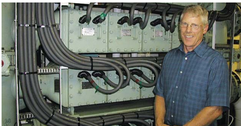
Tom Rausch, Marine Inspector, SLSDC, toured the ballast water treatment system called Electro-Clean that has been installed on the M/V Greenwing. Once IMO approval is given for this system, it will treat the ballast water on board in lieu of the vessel conducting ballast water exchanges.
