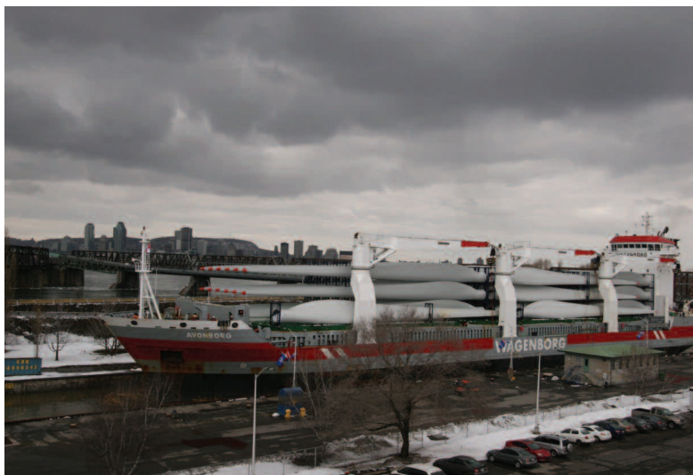
The Avonborg carries wind turbine components bound for Indiana through the St. Lambert Lock.
