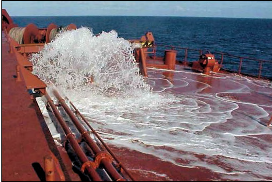
Figure 1: Water overflowing through a deck hatch on a commercial cargo vessel during flow-through exchange. (Photo courtesy of Smithsonian Environmental Research Center and the Great Lakes NOBOB Project).
