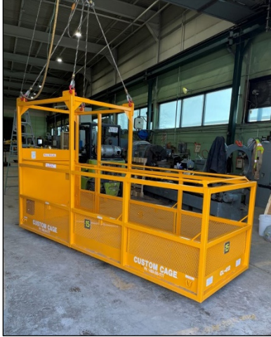
GLS's cantilever man basket for use in performing maintenance on the hands-free mooring system at both U.S. Seaway locks.
